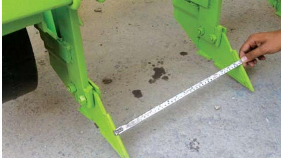
**Figure 25.** Distance between two alternate furrows
