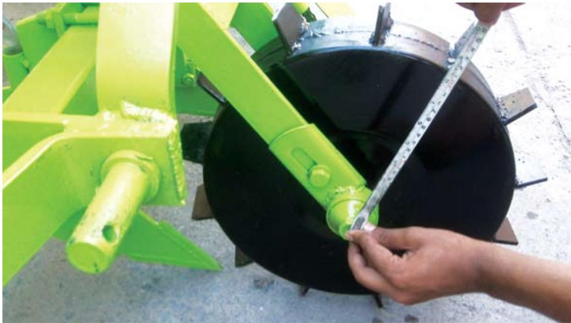
*Figure 24. Diameter of drive Wheel*
