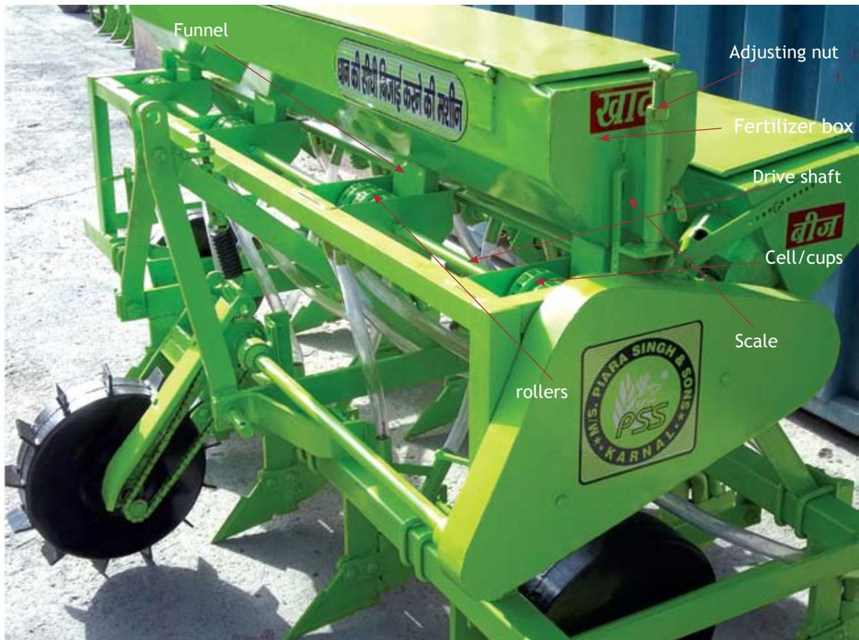
**Figure 15. Fertilizer metering components**
