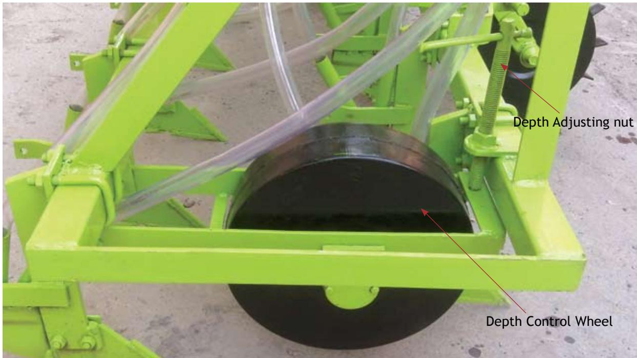
*Figure 19. Depth control wheel and its adjustment*
