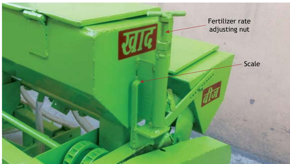
**Figure 16. Fertilizer rate adjustment**
