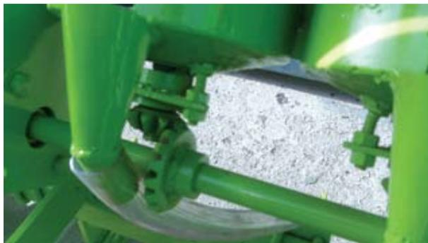
**Figure 21.** Power transmissions with Bevel gears
